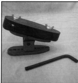
Pad ready to grind Toe Angle and Sides.
