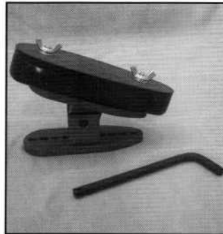
Pad ready to grind Toe Angle and Sides. Re-set fixture for Heel Angle.
